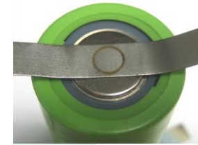
Copper battery tabs
